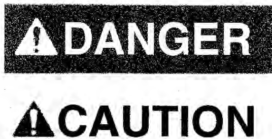
Figure 3 Examples of two signal word panels including alert symbol and color. Note that the DANGER panel is white print on red background and the CAUTION is black print on yellow background. Not shown is the WARNING panel, which is black print on orange background.
