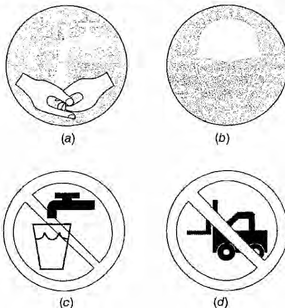
Figure 5 Examples of pictorial symbols conveying instructions/directions information: (a) wash hands; (b) wear hard hat; (c) do not drink water; (d) no forklifts in area.
