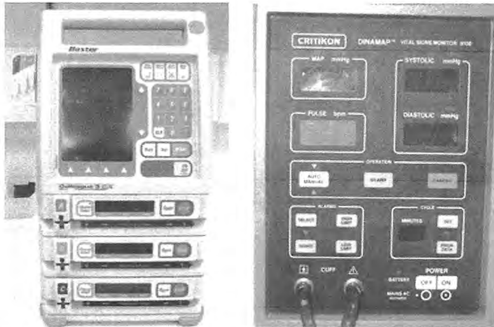
FIGURE 13.18 Labels should be placed close to the related controls, displays, ports, and so on to which they refer. These photos of medical devices show how the use of Gestalt principles can enhance the effectiveness of medical labeling.
