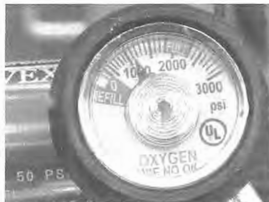
FIGURE 13.15 Avoid using curved text on labels, except as setting delimiters for rotary controls and display.
