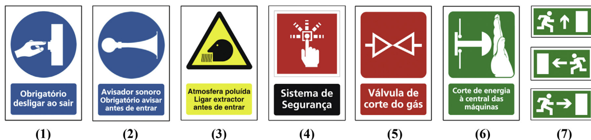
Fig. 5. Stimuli used in the experiment. Uncued signs (1–3): (1) music – mandatory to disconnect before leaving the room; (2) siren – mandatory to warn before entering; (3) air extractor – inhalation hazard, start air extractor before entering the room; cued signs (4–6): (4) security system; (5) gas valve; (6) cut-off energy to machinery room; and exit signs (7).
