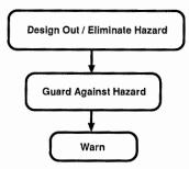
FIGURE 1.1. Hazard control hierarchy.
