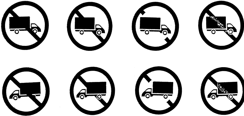
Fig. 2. Example NO TRUCKS Pictorial in the 8 slash type variations (over, under, partial and translucent) and orientation (I = left versus II = right).
